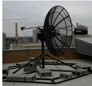
Figure 2: The Small Radio Telescope (SRT) on the roof of Sterling Hall at UW-Madison. Second SRT is located in Pine Bluff.
