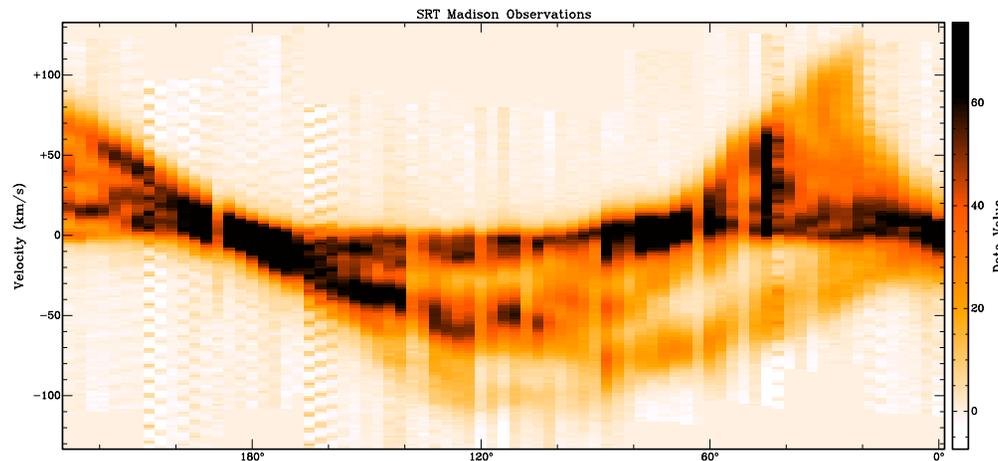
Figure 3: The I - Vr diagram, at b = 0 degrees and increment l from l = 0 to l = 231 degrees, obtained with the Small Radio Telescope.
