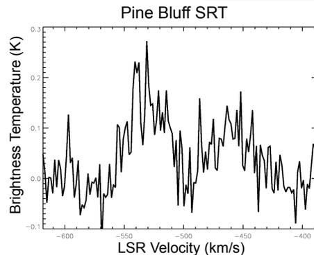
Figure 3. Approx. 70 minutes integration; averaged and corrected for telescope gain. We detect a peak centered at -525 km/sec where Andromeda is expected to be the brightest.
