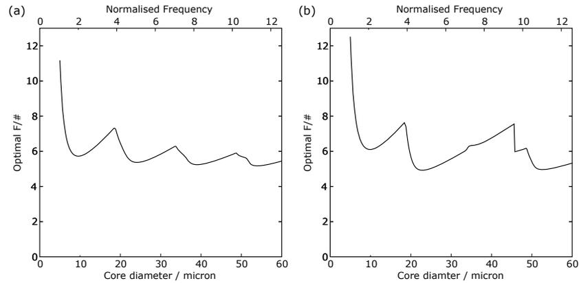
Fig. 2. Optimal focal ratio versus core diameter for an NA = 0.1 fibre at a wavelength of  $1.5\mu\text{m}$ . The focal ratio corresponding to maximum coupling efficiency is shown for (a)  $\alpha = 0$  and (b)  $\alpha = 0.2$ .
