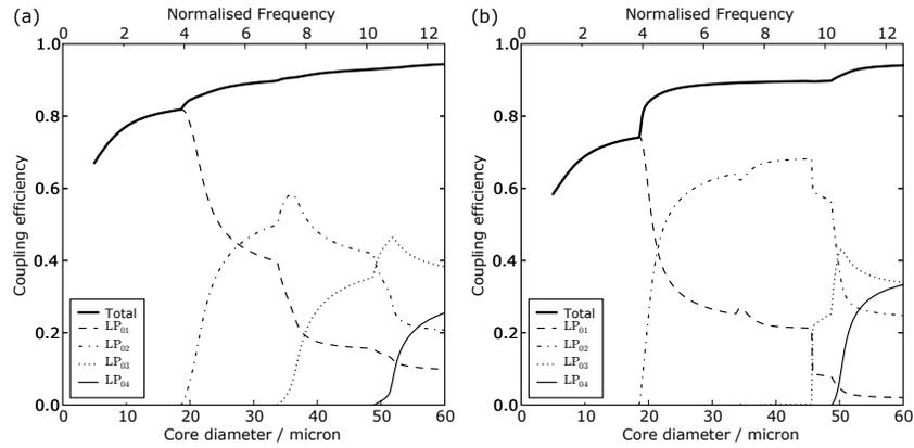
Fig. 1. Maximum coupling efficiency versus core diameter for an NA = 0.1 fibre at a wavelength of  $1.5\mu\text{m}$ . The overall coupling efficiency and the contributions from each fibre mode are shown for (a)  $\alpha = 0$  and (b)  $\alpha = 0.2$ .
