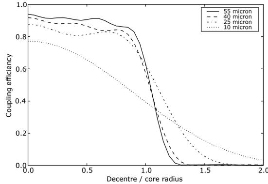
Fig. 4. Coupling efficiency versus decentering of the image centre from the fibre axis. Coupling efficiency is shown for  $NA = 0.1$  fibres with 10, 25, 40 and  $55\mu\text{m}$  core diameters at a wavelength of  $1.5\mu\text{m}$  and with  $\alpha = 0$ .
