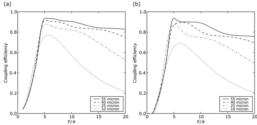
Fig. 3. Coupling efficiency versus focal ratio for an  $NA = 0.1$  fibre at a wavelength of  $1.5\mu\text{m}$ . Coupling efficiency is shown for core diameters of 10, 25, 40 and  $55\mu\text{m}$  with (a)  $\alpha = 0$  and (b)  $\alpha = 0.2$ .
