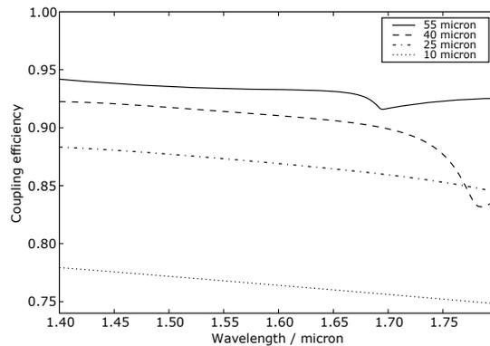
Fig. 5. Coupling efficiency versus wavelength for  $NA = 0.1$  fibres with core diameters of 10, 25, 40 and 55 $\mu\text{m}$ , and with  $\alpha = 0$ . For each diameter the focal ratio was fixed at the optimal value for a wavelength of 1.6 $\mu\text{m}$ .
