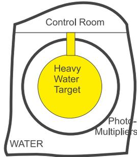
**Figure 8.** A schematic drawing of the SNO experiment. The neutrino target, 1000 tons of heavy water, is contained in an acrylic sphere, which is immersed in a light-water buffer to shield it from external radioactivity. Altogether 9500 photomultipliers are installed on a geodesic sphere surrounding the acrylic vessel.
